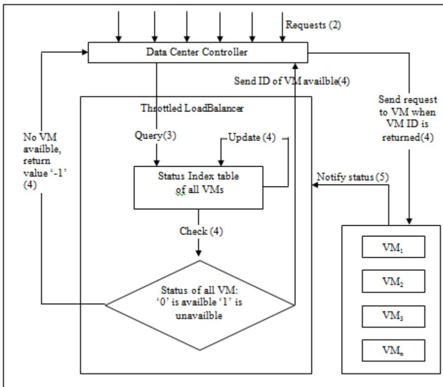
**Figure 1:** Throttled algorithm operation diagram
