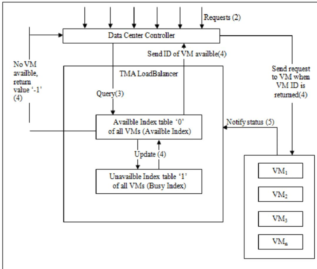
Figure 2: TMA operation diagram
